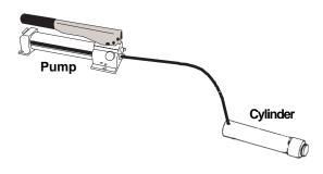
IMPORTANT: Some spring return cylinders, or rams, have a cavity in the rod which forms an air pocket. This type of cylinder or ram should be bled when positioned upside down or lying on its side with the port facing upward.
